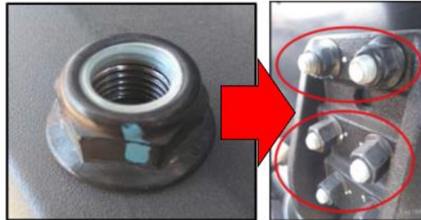
Gambar 4. 10 Alternatif Solusi Install with Plastic Nut
