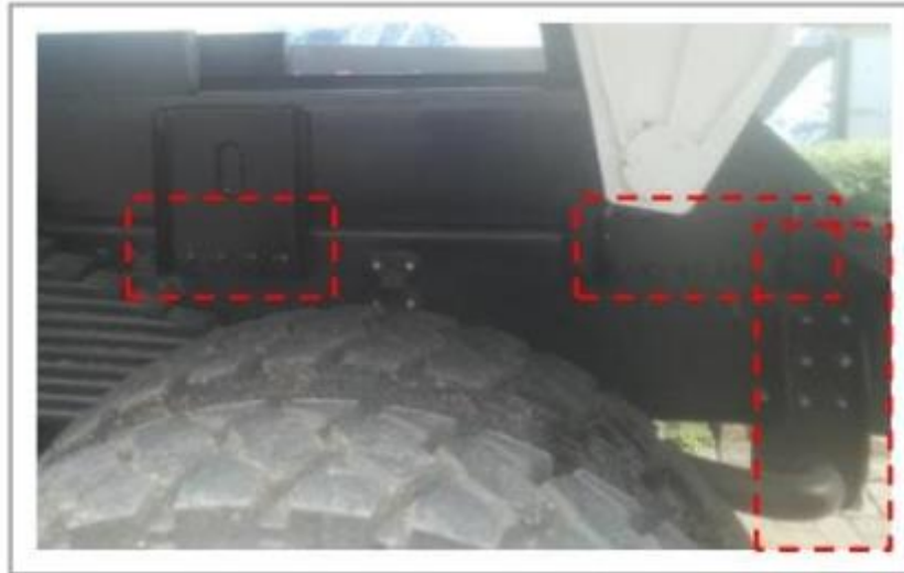
Gambar 4. 9 Lokasi Improvement Bolt Rear Stabilizer
