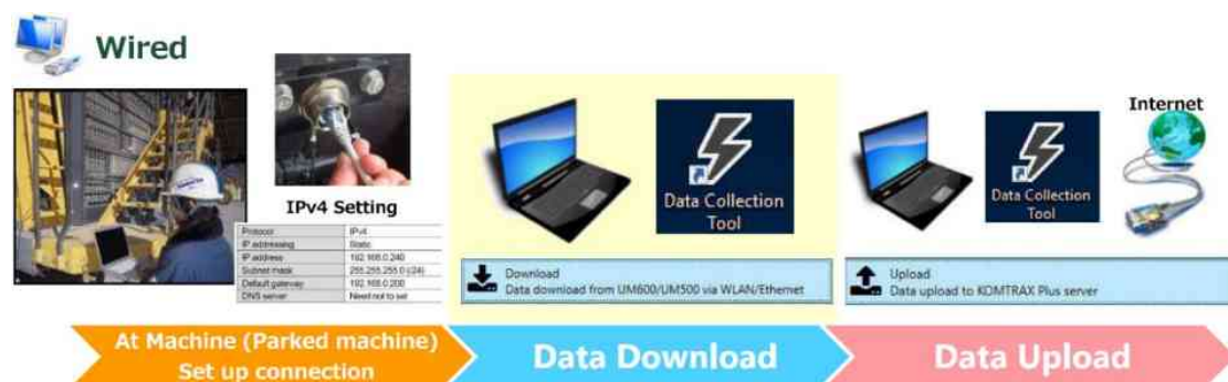
Figure 2.7 VHMS wired data downloading and processing.
