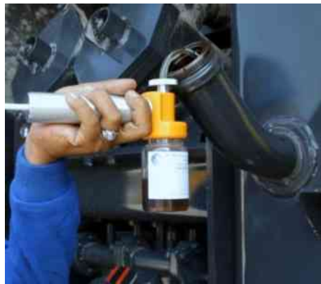
Figure 2.11 Hydraulic Oil Sampling of HD785-7
