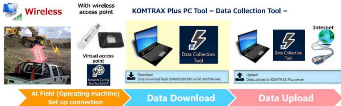
Figure 2.8 VHMS wireless data downloading and processing.
