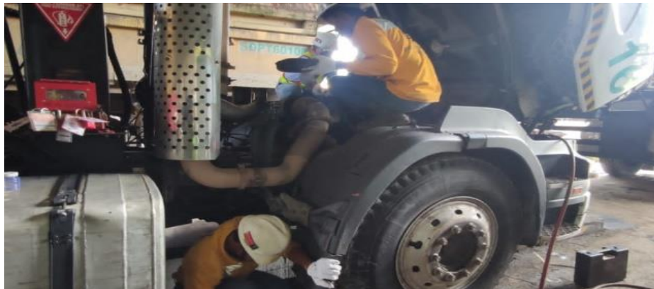
Gambar 4.15 Pelaksanaan Adjust Injector & Valve Clearance Engine scania R580
