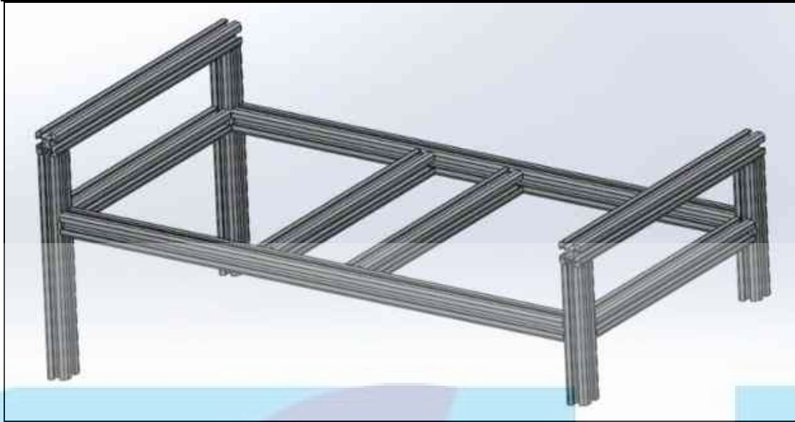
Figure 3.12 – Main structure made out of aluminum profile
