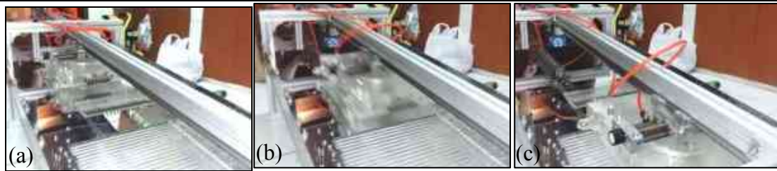
Figure 4.8 – The result for clamping mechanism: (a) initial, (b) advances, (c) final
