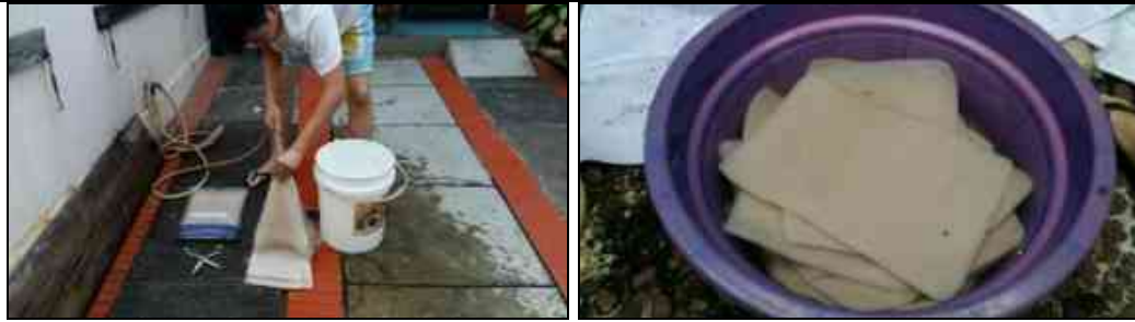
Figure 4.11 – The sample soaked in water to soften the texture
