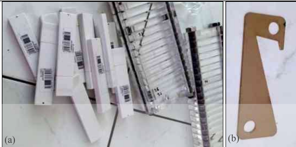
Figure 4.15 – The blades are (a) changed into paper cutters with (b) new jigs
