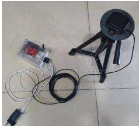
Figure 3-7 GPS-RTK2 as Base Station
