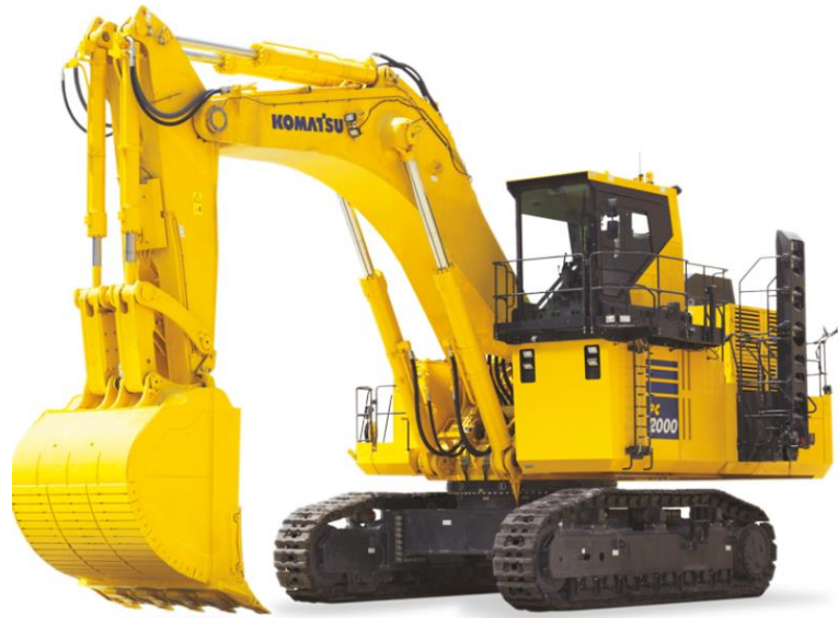
Figure 2. 2 Hydraulic Excavator PC2000
