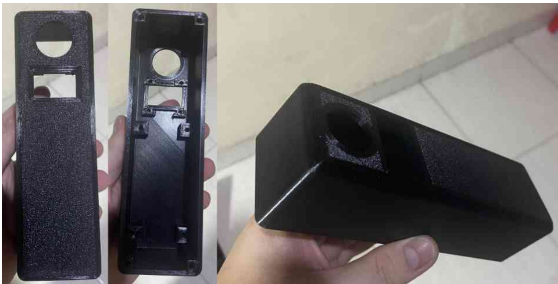
Figure 4.1 3D Printed PCB Enclosure
