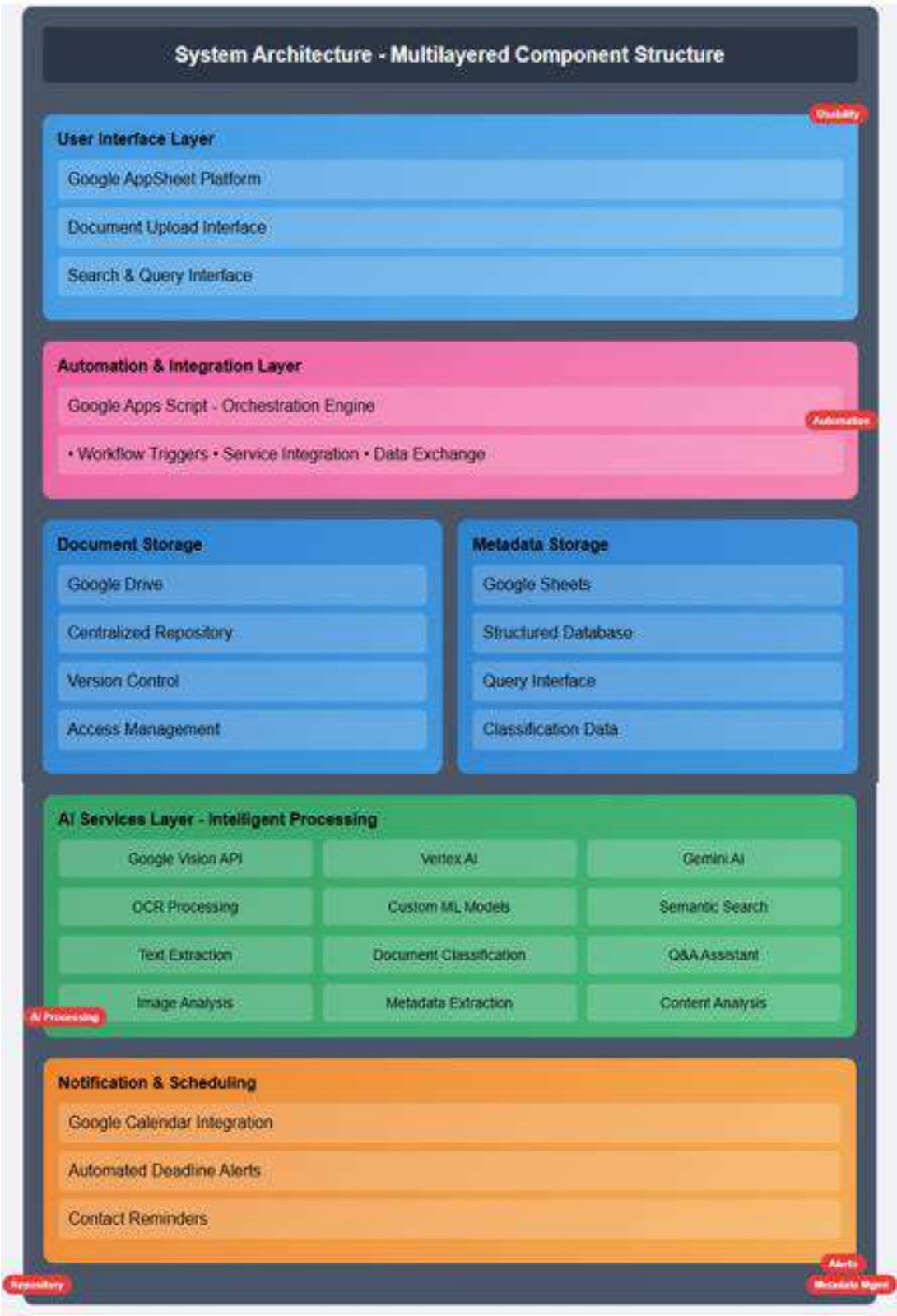
Figure 4.1 System Architecture Layers
