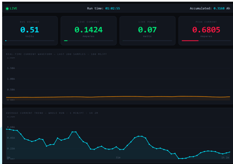
Figure 4.15: Dashboard interface illustrating the maximum solar current generation under direct sunlight, achieving a recorded peak of 0.68A
