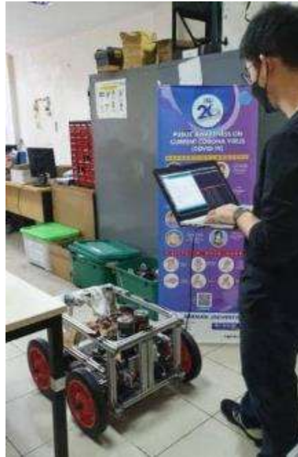
Figure 4-17 Robot Keyboard Teleoperation Test
