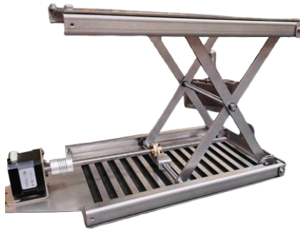
Figure 2.10 Scissor Lift with Lead Screw
