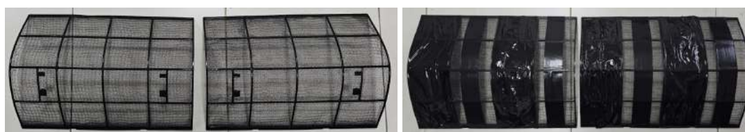
Figure 4.30 Initial Indoor Filter Condition, Blocked Indoor Filter Condition
