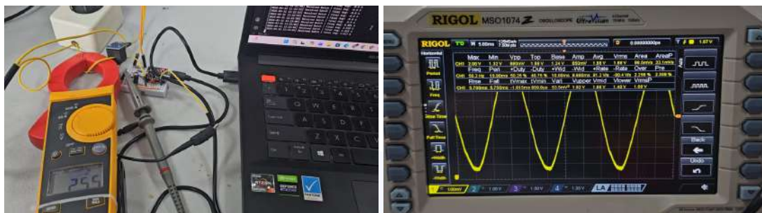
Figure 4.4 Current Sensor Testing with Fluke Meter and Oscilloscope
