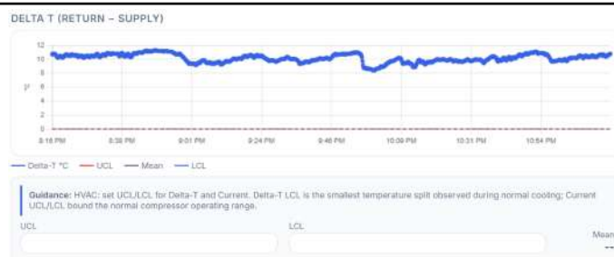
Figure 4.28 Baseline Setting Guidance for Split HVAC
