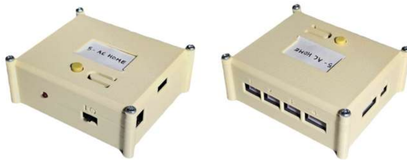
Figure 4.14 Printed Sensor Node Housing
