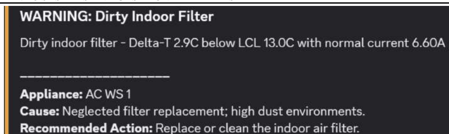
Figure 4.31 Generated Discord Indoor Filter Alert
