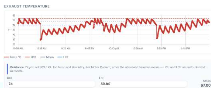
Figure 4.29 Baseline Setting Guidance for Gas Dryer
