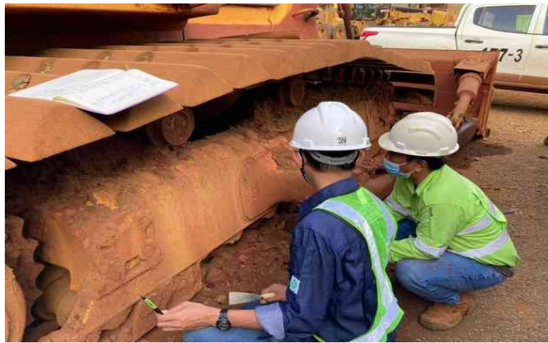
Figure 21. Undercarriage Inspection (P2U) program
