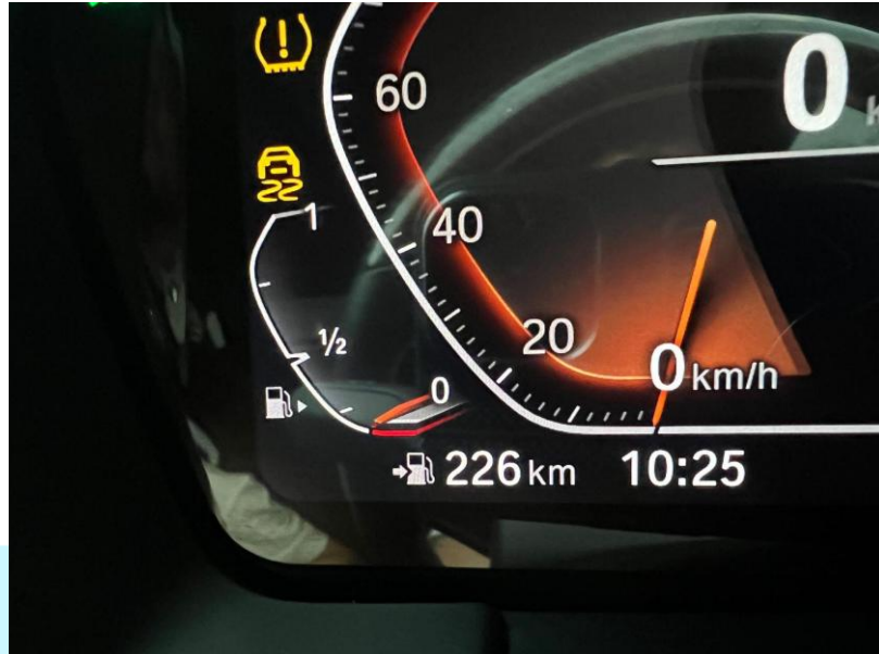
Figure A.4: The physical digital instrument cluster of the BMW Z4 during active testing. The physical fuel gauge indicates a remaining capacity slightly below the one-quarter mark.
