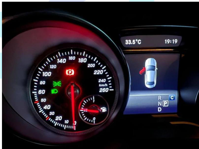
Figure A.7: The physical analog instrument cluster of the Mercedes CLA during active testing. The physical fuel gauge indicates a remaining capacity slightly above the halfway
