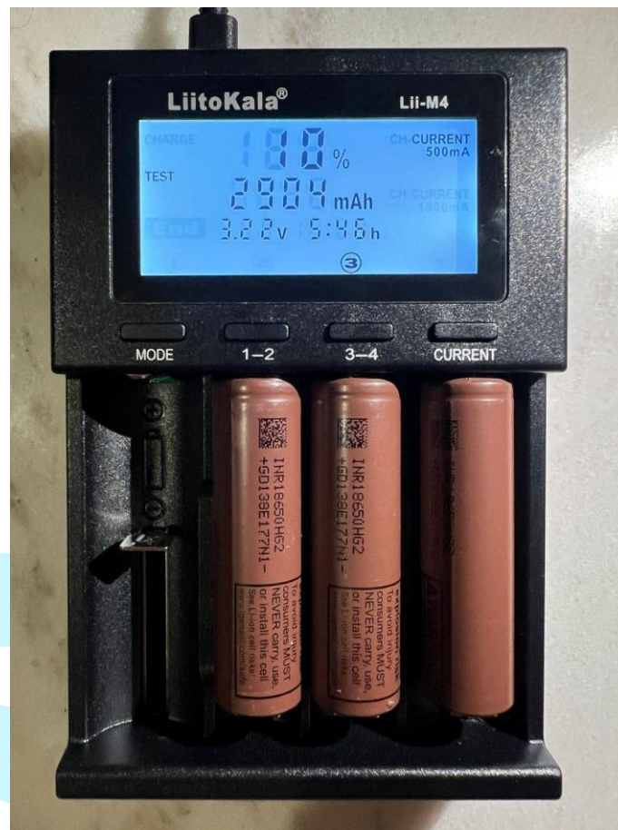
Figure A.2: Physical capacity validation of an individual 18650 lithium-ion cell using a LiitoKala Lii-M4 battery analyzer, confirming a tested capacity of 2904 mAh.
