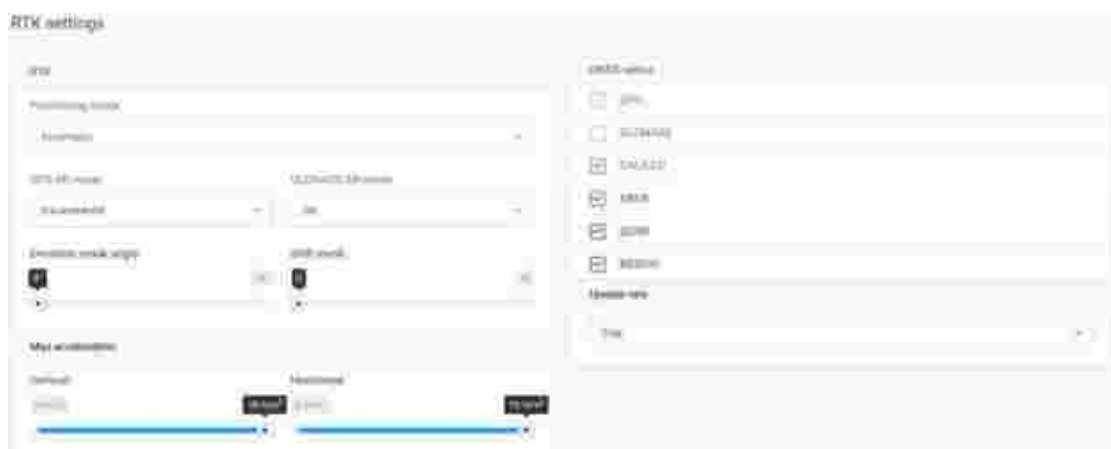
Figure 3.11 ReachView Rover Receiver RTK Settings
