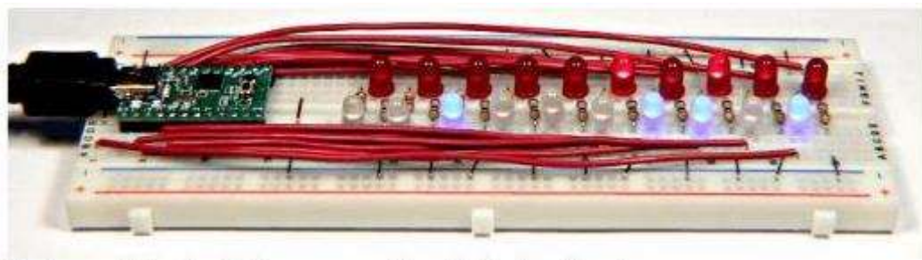
Figure 2-10 Teensy Usage on Solderless Breadboard
