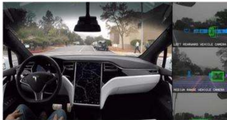
Figure 2-32 Camera as Vision Sensor on Tesla
