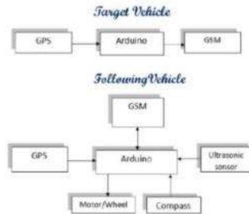
Figure 2-40 Test Robot Block Diagram (Existing Research 1)
