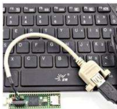
Figure 2-14 USB Host port on Teensy 4.1
