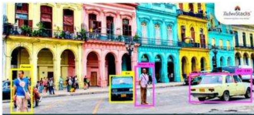
Figure 2-28 Incompleteness of YOLO to Identify Small Objects
