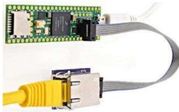
Figure 2-15 Ethernet Kit on Teensy 4.1
