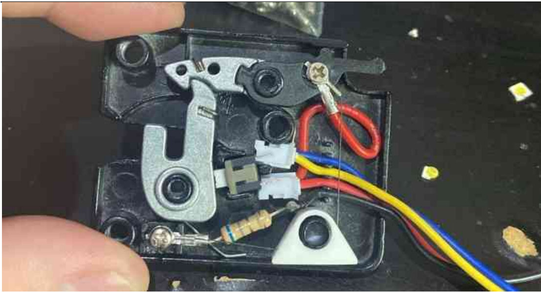
Figure 3.10 Lock Body Internal Mechanism
