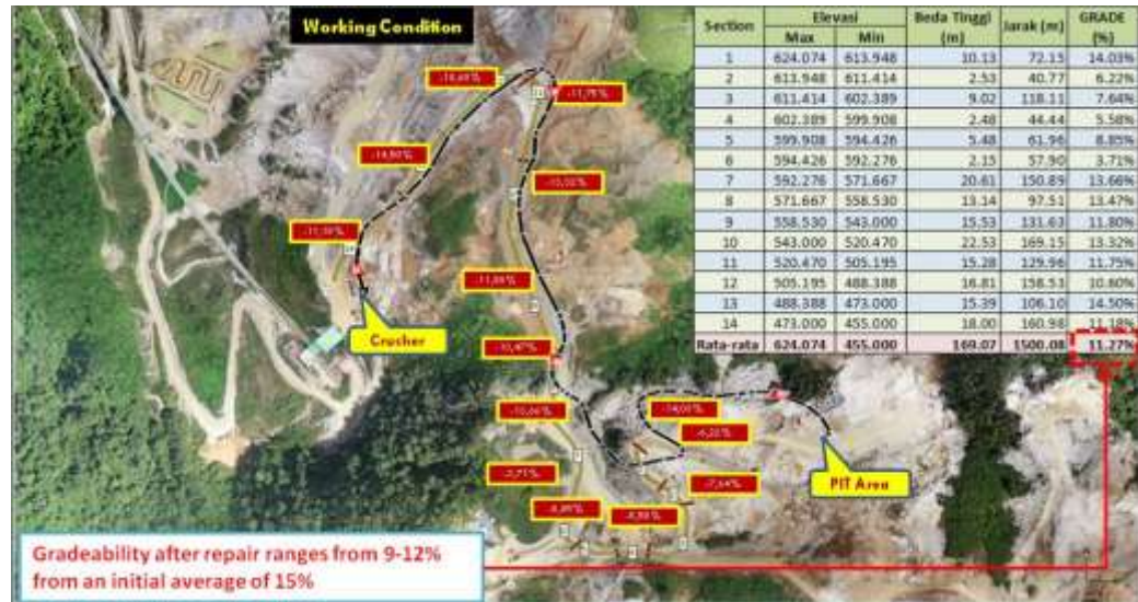
Fig 4.1 Final Gradability at Project-X after Cutting
